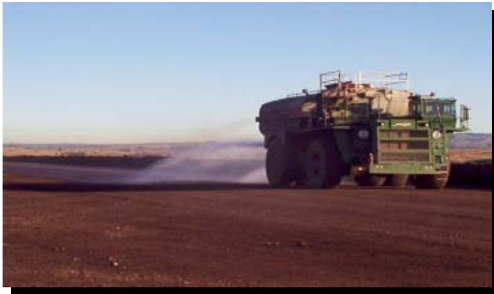
A water spreading truck operating at the Spring Creek Coal Mine in Montana. The truck is spreading water to minimize fugitive dust.
