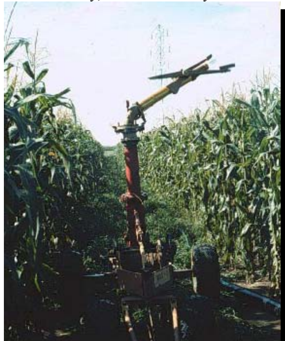
Big Gun Irrigation System is a high pressure, large capacity nozzle that can be used to throw CBM water in a 175 to 300 foot radius.
