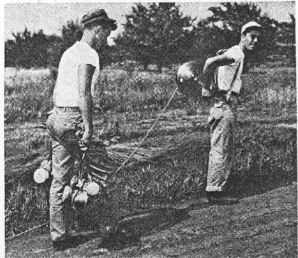
Surveying team measuring traverse stations where geophones are placed.
