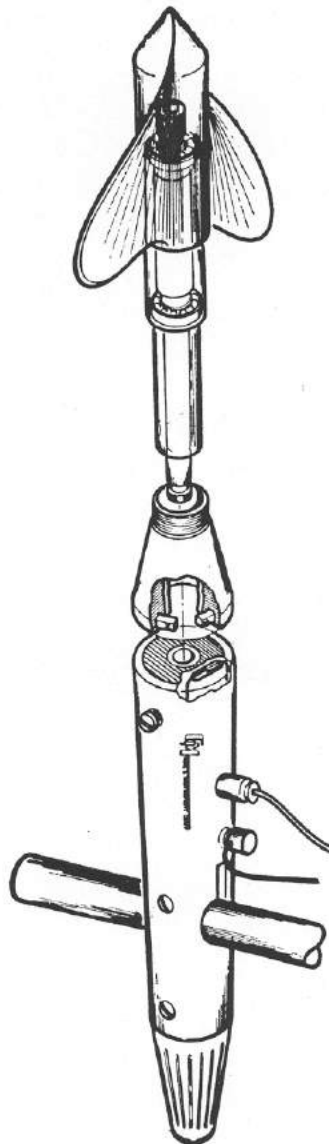
Magnetic-type flowmeter for down-hole current measurements.
