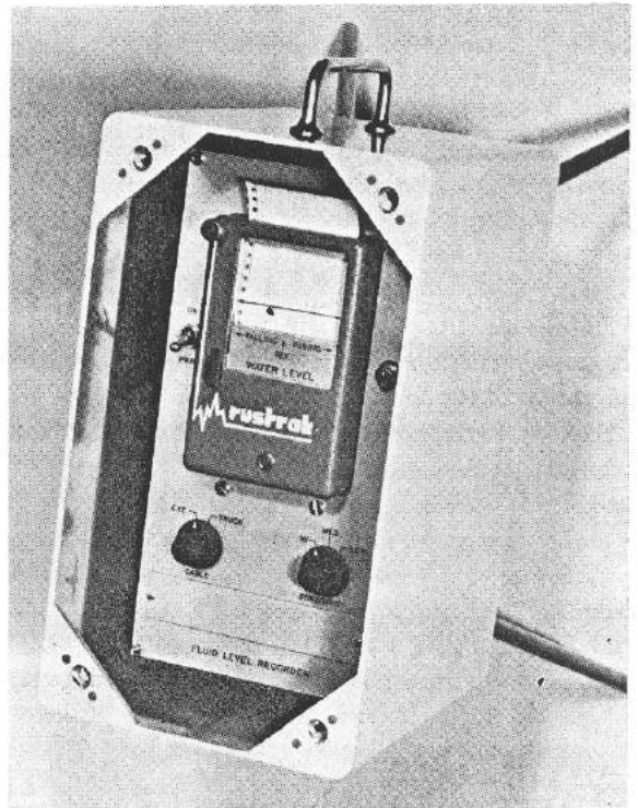
Continuous water level recording monitor with water-proof housing.
