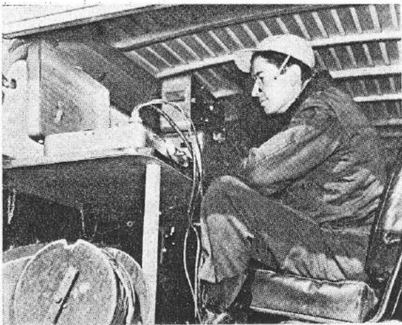
Control monitor unit inside recording vehicle which will receive seismic information from geophone traverse stations.
